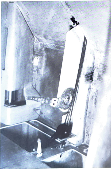
View of center console showing CZRTH Roll Trim Handle mounted on instrument panel, VECG Throttle Quadrant Assembly, and CZLB-13 Landing Brake Handle extended.
