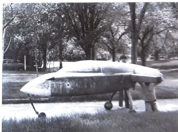
Continuous smooth curve from front of bubble to prop.
