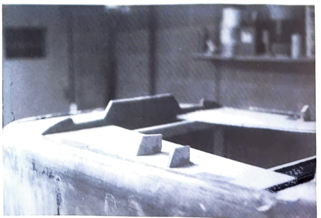
Spreader blocks for plexiglass bubble.
